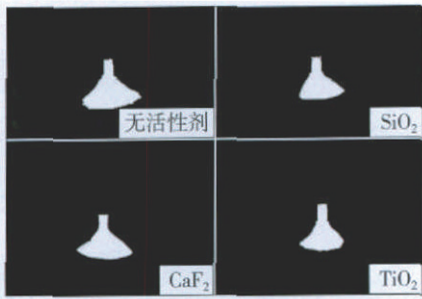
图4 不同活性剂下激光-TIG复合焊电弧形态二值化图 Fig.4 Arc shapes binarization of laser-TIG hybrid welding with different fluxes
